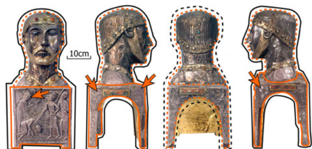
Figure 8: Mapping of the tarnish on the reliquary head using cathodic voltammetric plots. The tarnish due to AgCl and Ag 2 S are respectively underlined in orange and black: major (solid lines) and minor (dashed lines) (© Atelier de l'Abbaye de Saint-Maurice).
