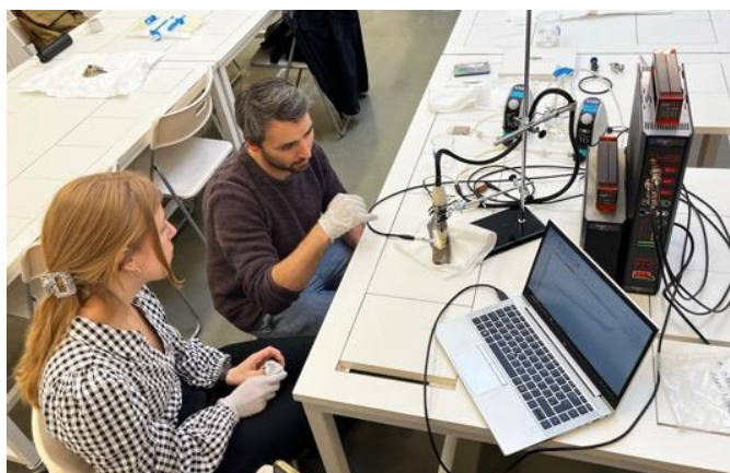
Set-up for analyzing corrosion products and their reduction with the Pleco® and a potentiostat. ©Eva Menart
