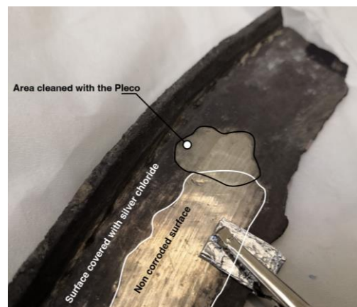
Detail of fragment no. 3 after silver chloride reduction with Pleco®. ©Romain Jeanneret
