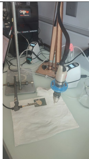
Fig. 11: The setup for tarnish removal using the Pleco instrument
