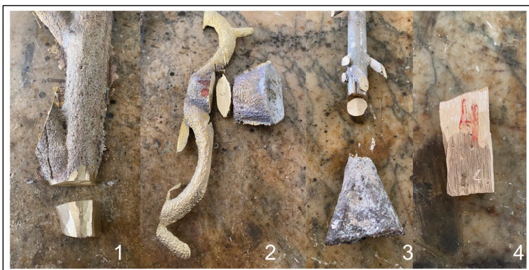
Fig. 2. Samples studied during the ENDLESS Metal STSM, after cutting them from the reverberation tubes. Samples 1 and 3 correspond to casts from the year 2023, sample 2 is from a sculpture cast in 2022 and sample 4 corresponds to a sculpture cast in the 1970 decade. © Pablo General.
