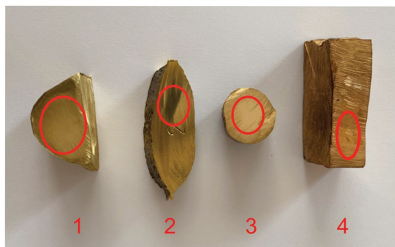
Fig. 3. The surfaces of the samples were polished (marked with the red circles) to improve the measurement reproducibility with DiscoveryMat. © Pablo General.
