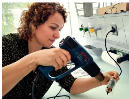
Figure 1. First steps in assembling a new Pleco (left) and making the envelope of Pleco from the heat-shrink tube with a heat gun (right).
