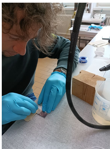
Figure 16. Burnishing the coupon with cotton cloth, © Degriigny Christian.
