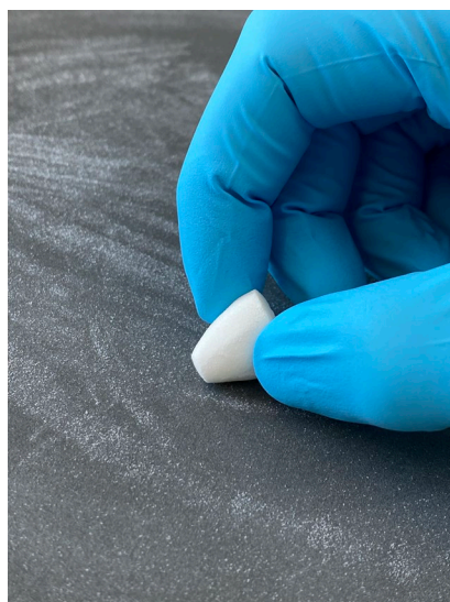
Figure 14. Dry pad worked by abrasive paper, © Ricotta Nicola.
