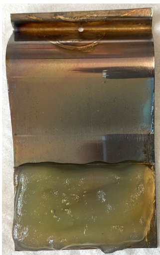
Figure 11. Coupon with Na 2 -EDTA gel made alkaline, © Ricotta Nicola.
