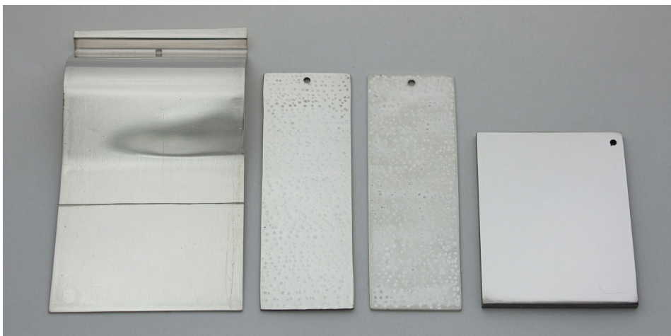
Figure 4. Coupons before artificial tarnishing, from left to right: curved and mirror; flat, punched and mirror; flat, punched and matte; flat and mirror, © Ricotta Nicola.
