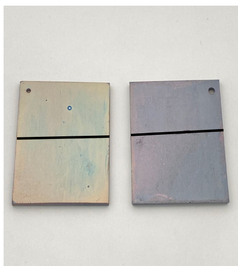
Figure 7. Left coupon tarnished for 1h and right coupon tarnished for 48h. Above black line: untreated area and below: Na 4 -EDTA treated area, © Ricotta Nicola.
