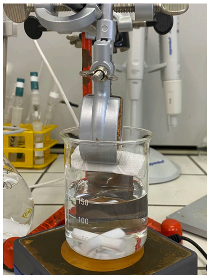
Figure 9. Coupon half immersed inside Na 2 -EDTA made alkaline, © Ricotta Nicola
