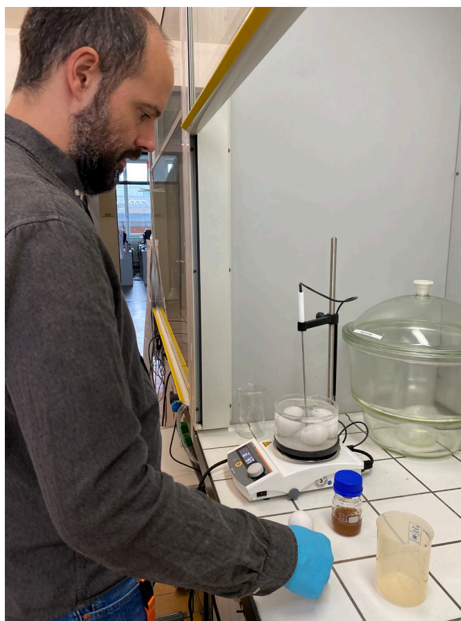
Figure 5. Jorge Gonzalez Frutos during the preparation of boiled eggs for tarnishing coupons, © Ricotta Nicola.
