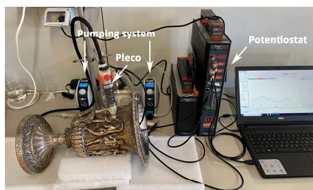
Figure 2. Electrolytic setup to obtain LSV plots of the body of the Valadier cooler using the Pleco
